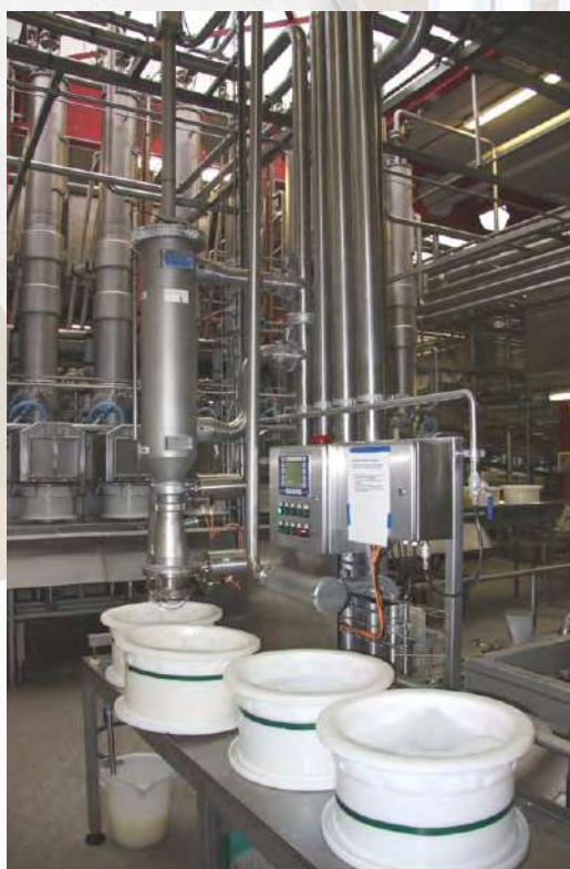
Auto-line® XLE for filtration of curd particles from whey after cheese forming
