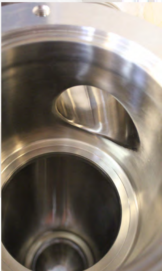
Filter housing polished to Ra 0,8 micron
