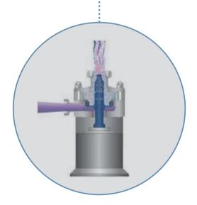
The UTL is a single-stage dispersing machine for the production of emulsions and suspensions with a coarse or medium particle size and a narrow particle size distribution. There are numerous rotor-stator variants, enabling the adaption of the machine to the respective application.
