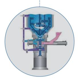
The DBI is a high-performance mixing and dispersing machine for the production of finest emulsions and suspensions. To enable this, both solid and liquid additives are incorporated into a base liquid.
