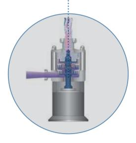
The DR/DRS is a high-shear dispersing machine for the production of microemulsions and ultra-fine suspensions, for wet milling and for dissolving processes. Whilst the production machines of type DR are operated with standard circumferential speeds of approx. 23 m/s and 3 tools, with the magic LAB®, the fast-running variant of type DRS with circumferential speeds of up to 40 m/s and 2 tools in series can also be simulated.
