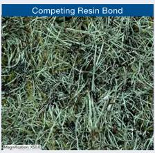
The 50x magnification images of two clean filters demonstrate how the **ECO-RBU** achieves such incredible open area (void space) improvements compared to traditional resin bonded filters.
