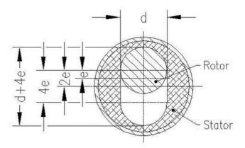
The dimensions at the stator enable the rotor to revolve in it without any play. Consequently the propulsion height—O does not permit any back-flow. If the propulsion height is greater, the QSp increases linearly. Whereupon the dimension tolerances of the stator and the rotor as well as the elasticity of the stator are decisive. The viscosity and temperature of the fluids also have a great impact on the situation.
