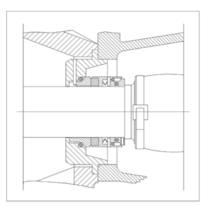
Mechanical seal single-acting, independent of the direction of rotation
