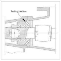
Standard gland packing with soft packingand flush ring for strongly abrasive, cristalline media
