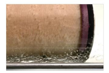
The new XtreamPhase, Series 110XP single stage horizontal coalescers take liquid separation to the next level of performance. The 110XP utilizes high flow style coalescer cartridges that flow inside-tooutside. The cartridges include a handled end cap with PECOSeal<sup>™</sup> technology so there is no need for tools when sealing making them a safe, user friendly choice while also reducing maintenance time and money.
