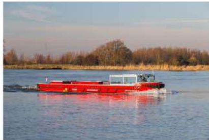
Low profile design to pass underneath bridges
