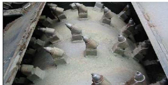
Road grinding cutting depths may go up to 12 inches (30.48 cm) deep and widths up to 72" (182.88 cm) wide
