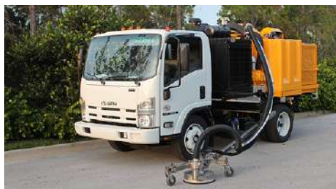
Medium Duty surface preparation truck equipped with Logan LC-211 Bell Housing PTO powered by a 200 HP Diesel engine.
