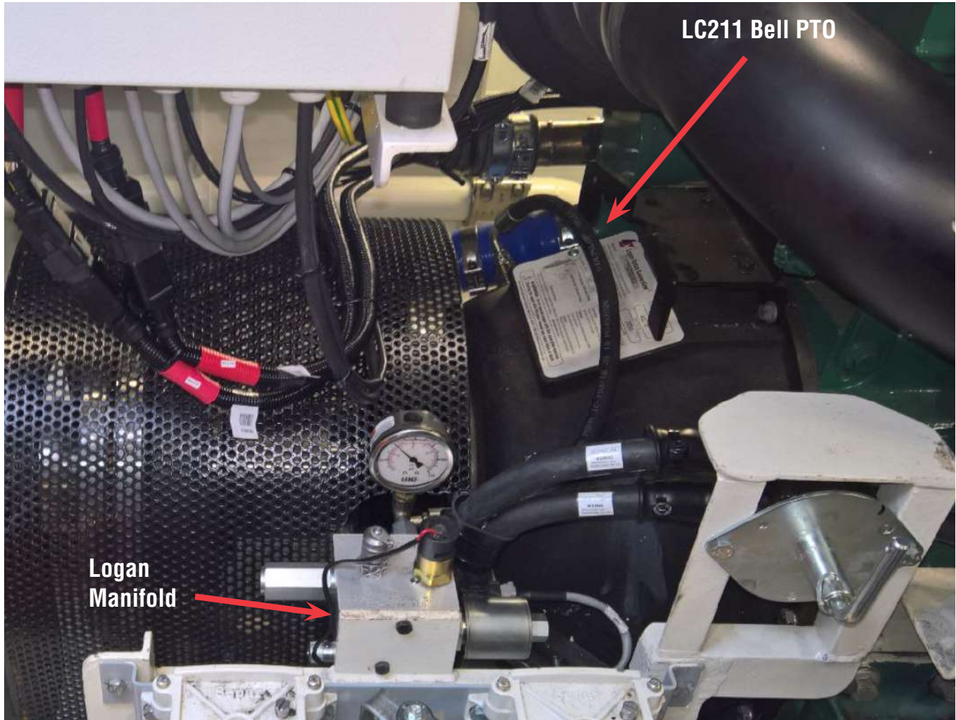
Logan LC-211 Bell Housing PTO transmits 963 lb.ft. (1350Nm) @ 200 psi. Logan 034 series Softstart™ manifold controls pressure to the clutch.
