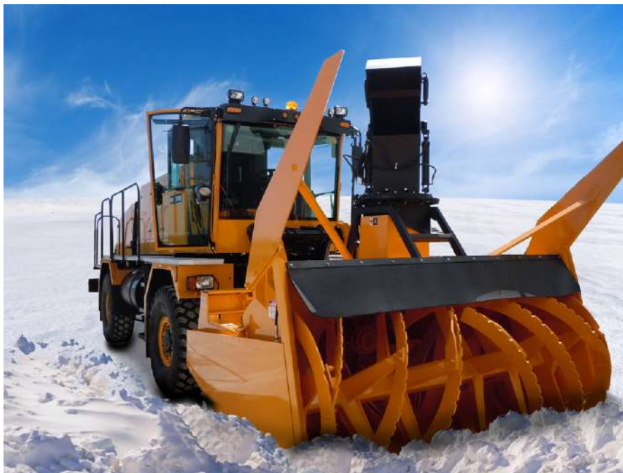
This Airport 700 HP Snow Blower is equipped with a Logan LC-318 Bell Housing PTO and is capable of clearing a 120" wide path of snow, moving 6000 tons of snow per hour
