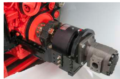
Logan Front PTO's act as connect/disconnect for auxiliary pumps
