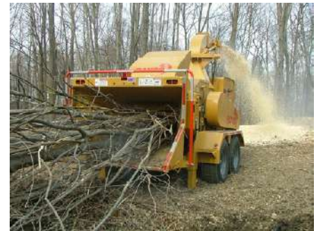
Feed / discharge system has 20" (50.8 cm) chipping capacity
