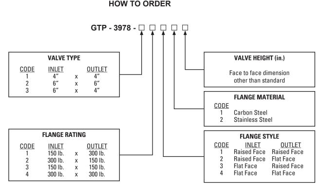
**EXAMPLE:** GTP-3978-23126 is an emergency valve as follows: 6" x 6" valve type, 150 lb. x 150 lb. flange rating, raised face flanges, stainless steel, with a valve height of 6 inches.
