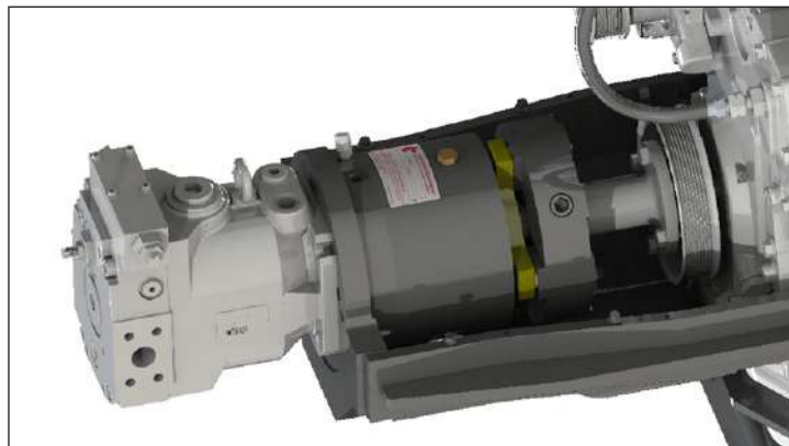
Logan 600 Series transmits 741 lb. ft. of torque (1004 kW) @ 100 psi (7 bar) / 1084 lb. ft. (1469 kW) @ 140 psi (9.5 bar). Max engagement speed is 1800 RPM. Clutch shown with cover plate removed.
