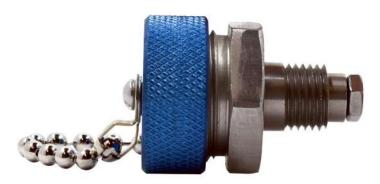
Made entirely of stainless steel, these couplers are fully interchangeable with Flight Refueling models, as well as those available from A. Searle & Co.. Because we make the caps of aluminum, there is no possibility of thread galling as in other brands when the coupler is also aluminum. We used the Gammon tapered gland O-ring seal principle that has proven to be astonishingly reliable for the last 50 years in the Jet Test QD®.
