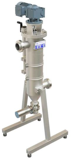
The benefit of the constant scraping is, that the filter can handle large amounts of dirt. The flow through the filter is continuous during scraping which means that the filter can work continuously and the flow is not interrupted.
