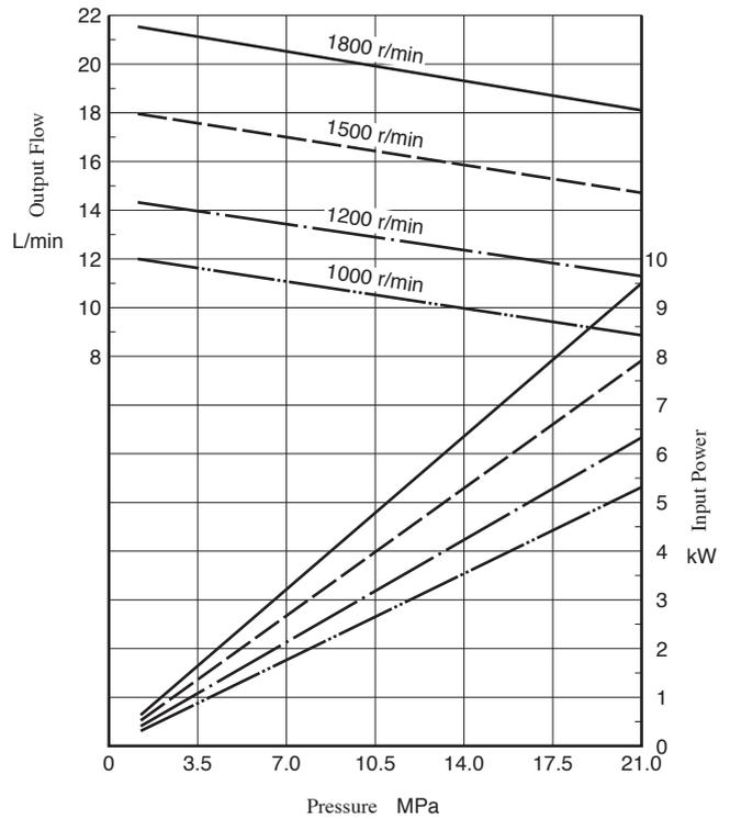
**Pressure, Output Flow, and Input Power**
