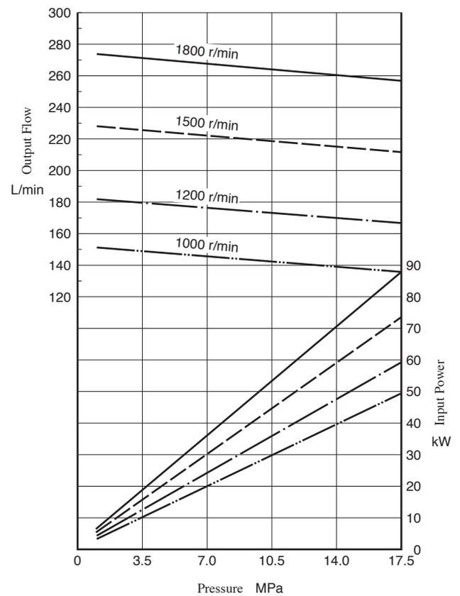
**Pressure, Output Flow, and Input Power**
