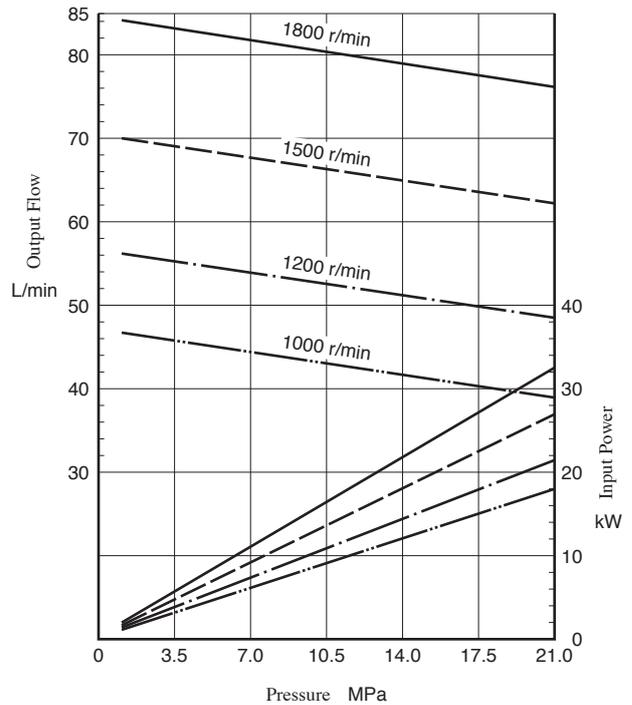
**Pressure, Output Flow, and Input Power**
