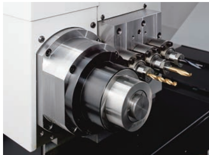
U121B (Rotary tool on the opposite tool post)
