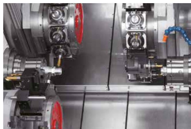
Simultaneous complex machining with three turrets
