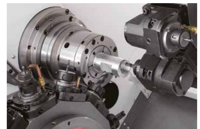
Simultaneous complex machining with two turrets
