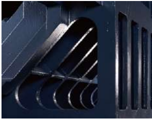
Thick ribs imparting high rigidity
