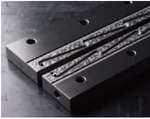
Scraped face of a hand scraped box slideway
