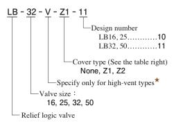
★Use high-vent pressure types if the shifting time from unloading to on-loading is reduced.
