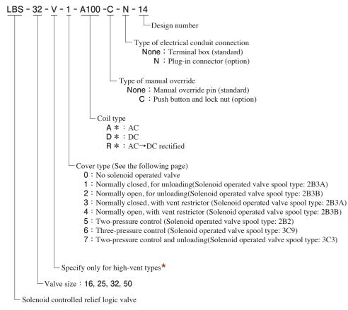
$\star$ Use high-vent pressure types if the shifting time from unloading to on-loading is reduced.
