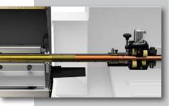
The continuously oil-flooded guide channel guarantees the highest level of guide properties seamlessly right up to the spindle.
