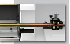
The continuously oil-flooded guide channel guarantees the highest level of guide properties seamlessly right up to the spindle.
